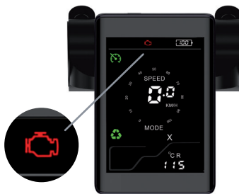
The motor has reached the overheating protection limit.
